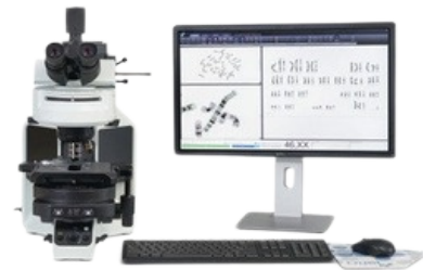
Manual capture with workstation with Karyotype and FISH analysis software
