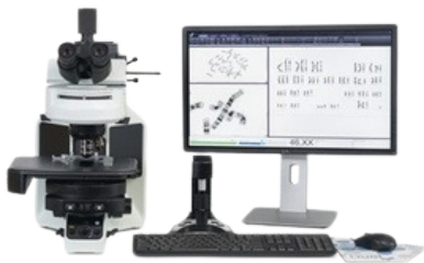
Manual capture workstation with Karyotype and FISH software equipped with motorized stage for easy metaphase location
